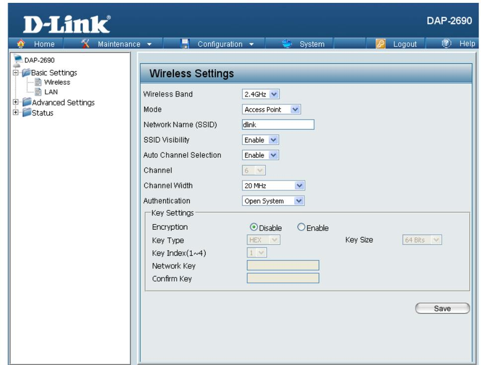
**Channel Width:** Allows selection of the channel width you would like to operate in. **20 MHz** and **Auto 20/40 MHz** allow both 802.11n and non-802.11n wireless devices on your network when the wireless mode is Mixed 802.11 b/g/n in 2.4G and Mixed 802.11 a/n in 5G. When the channel width is set to **Auto 20/40 MHz**, then 802.11n wireless devices are allowed to transmit data using 40 MHz.
