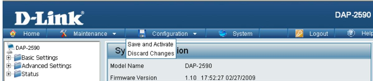
The drop-down Configuration menu allows users to save the current changes and reboot the DAP-2690 by clicking "Save and Activate".
