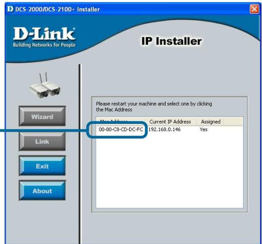
The IP Installer will now show a MAC address of the **DCS-2000** and an IP Address (which may or may not be correct depending on what you have your **DCS-2000** connected to.) If you have a DHCP\* server on your network, there will be a valid IP Address displayed here.
