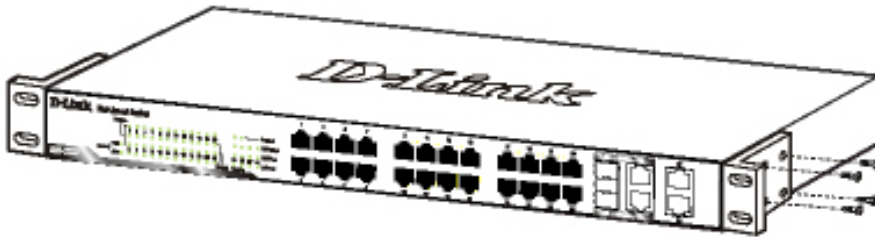
Figure 2 – Attach the mounting brackets to the Switch
