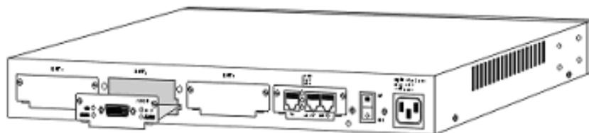
5. Push the module into place until the edge connector is securely seated in the connector on the motherboard. Ensure that each of the module's captive screw lines up with its corresponding hole in the chassis.
