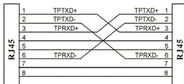
**Note:** The color code of the twisted-pair cable connection should comply with EIA/TIA 568A/B standard.
