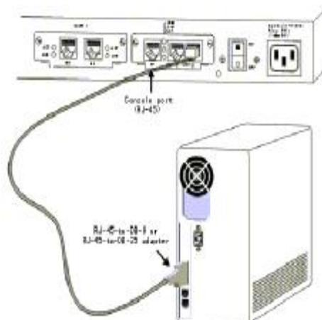
The pin details of the Console port is given in the following table:
