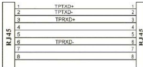
When connecting the DI-1750 Router directly to Ethernet port of single host computer, a UTP cross-over cable can be used. Thus you can eliminate the Fast-Ethernet Hub/Switch in the connection example above. But, when you need to connect more than one computer to the router, you must use an Ethernet Hub or switch. The illustration of the UTP cross-over connection is showed as following:
