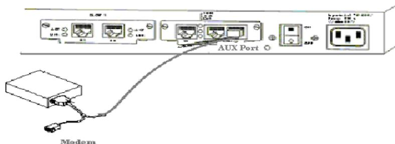
The auxiliary cable, DRC-0011 is used to connect the AUX Port with an external asynchronous modem. One end of the DRC-0011 cable is a standard RJ45 eight pin connector and the other end is DB25 and DB9 female connector. The RJ45 connector gets connected to the AUX Port of the router and on the other end you choose one from DB25 or DB9 according to the requirement of asynchronous serial port of Modem. The pin connection of the AUX cable DRC-0011 is showed in the following figure.
