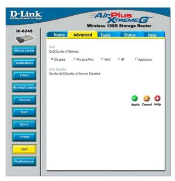
QoS or Quality of Service is used to allot bandwidth and priority from the router. To allot bandwidth per port on the router, click the **QoS Bandwidth** radio button and configure the parameters. QoS may be configured per **Physical Port**, **MAC address**, **IP address** or specified application. See the following explanation for more detailed information on each type of QoS setting.
