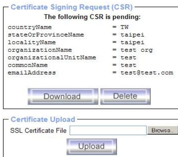
Figure 6-24. SSL Certificate Upload
