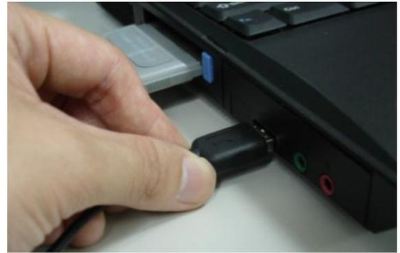
**Note:** The D-Link USB Phone Adapter **MUST** not be connected to a bus powered USB hub.
