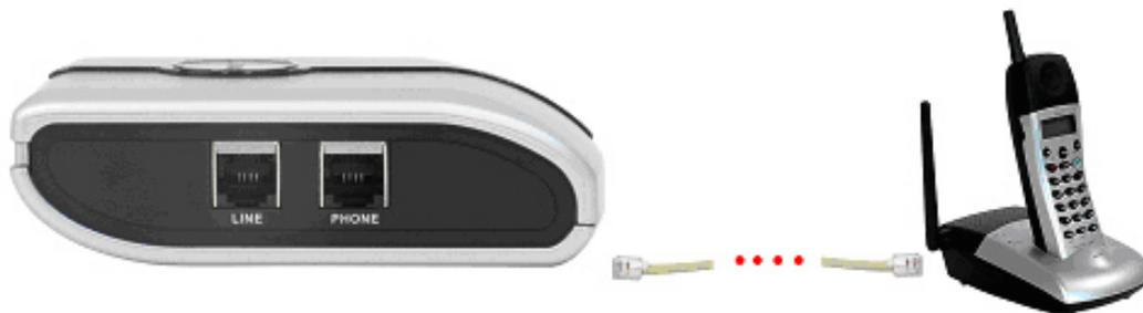
Connect a telephone cable between the DPH-50U **Line** port and a wall jack as shown below. Note that this is only required for making regular phone calls or for forwarding Skype calls to your mobile (or other off-site) phone or for toll bypass applications.
