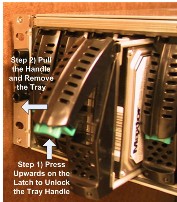
Figure 3-2 Drive and Tray Removal
